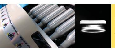
The underside of the curl, a likely place for a defect, is an extreme challenge to inspect. The Genius system achieves it, together with wall and neck-area inspections that help prevent defects from causing costly filler and consumer issues.
